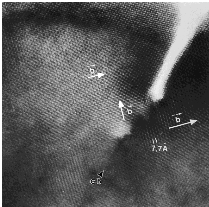
Figure 5. Enlarged image of the LT phase. Note the relationships between 2 in-plane parameters showing a grain boundary. The position of the heavy cations are imaged as bright dots.
